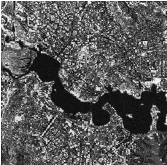
Figure TK-13: Land-water area of Canberra, Australia, viewed in the near-infrared band only. Note that the water appears black.
